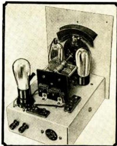
The super-regenerator which receives amateur and television signals on wavelengths from 3.7 to 7.2 meters—and how!
