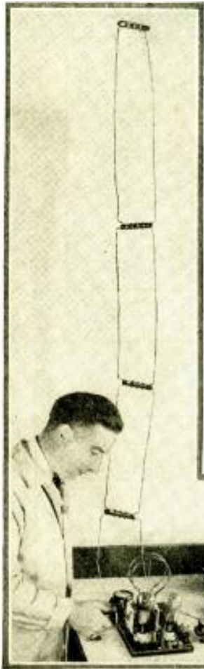
The five-meter phone transmitter set up and connected to aerial, data on which appears herewith.
