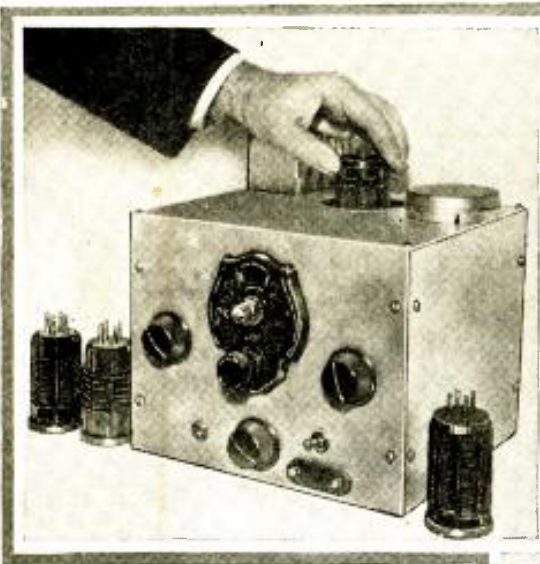
Above—The operation of removing one of the "plug-in" coils is shown clearly above. Many experts prefer the "plug-in" type of short wave receiver, and so here is a set that will appeal to them. After the coil has been put in place a metal cap covers the opening and thus completes the "shielding".
